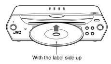
To insert an 8-cm disc, insert it into the center of the disc slot.
